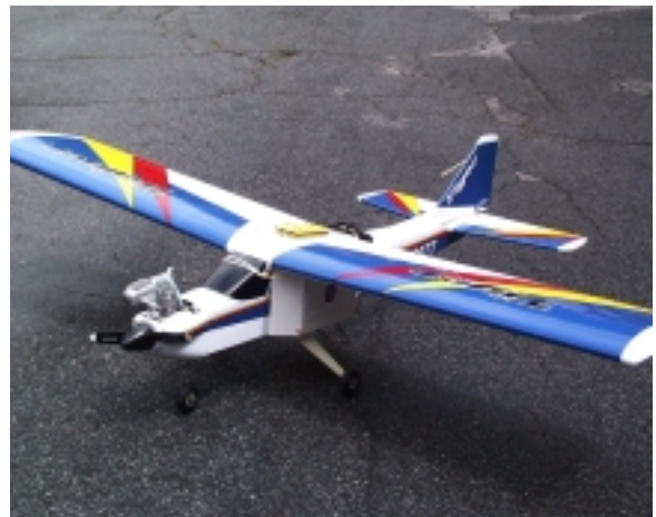
Figure 1. Low cost aerial vehicle, with avionics mounted above wing (GPS receiver), and in boxes on the sides of the fuselage (computer and battery)
